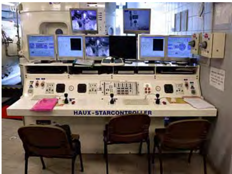
Above: a control console for the de-compression chambers.
